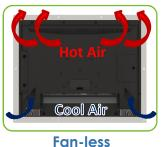
Aluminum Die-casting Housing design allows heat to escape.
