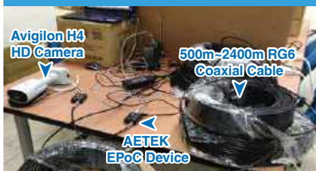
EPoC 1 - to - 1 Test
