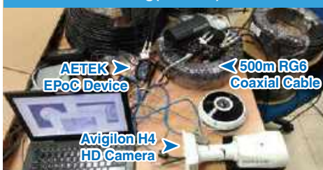
EPoC Ring(Failover) Test
