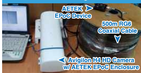
EPoC Camera Housing 1 - to - 1 Test
