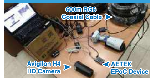
EPoC Daisy-Chain Test
