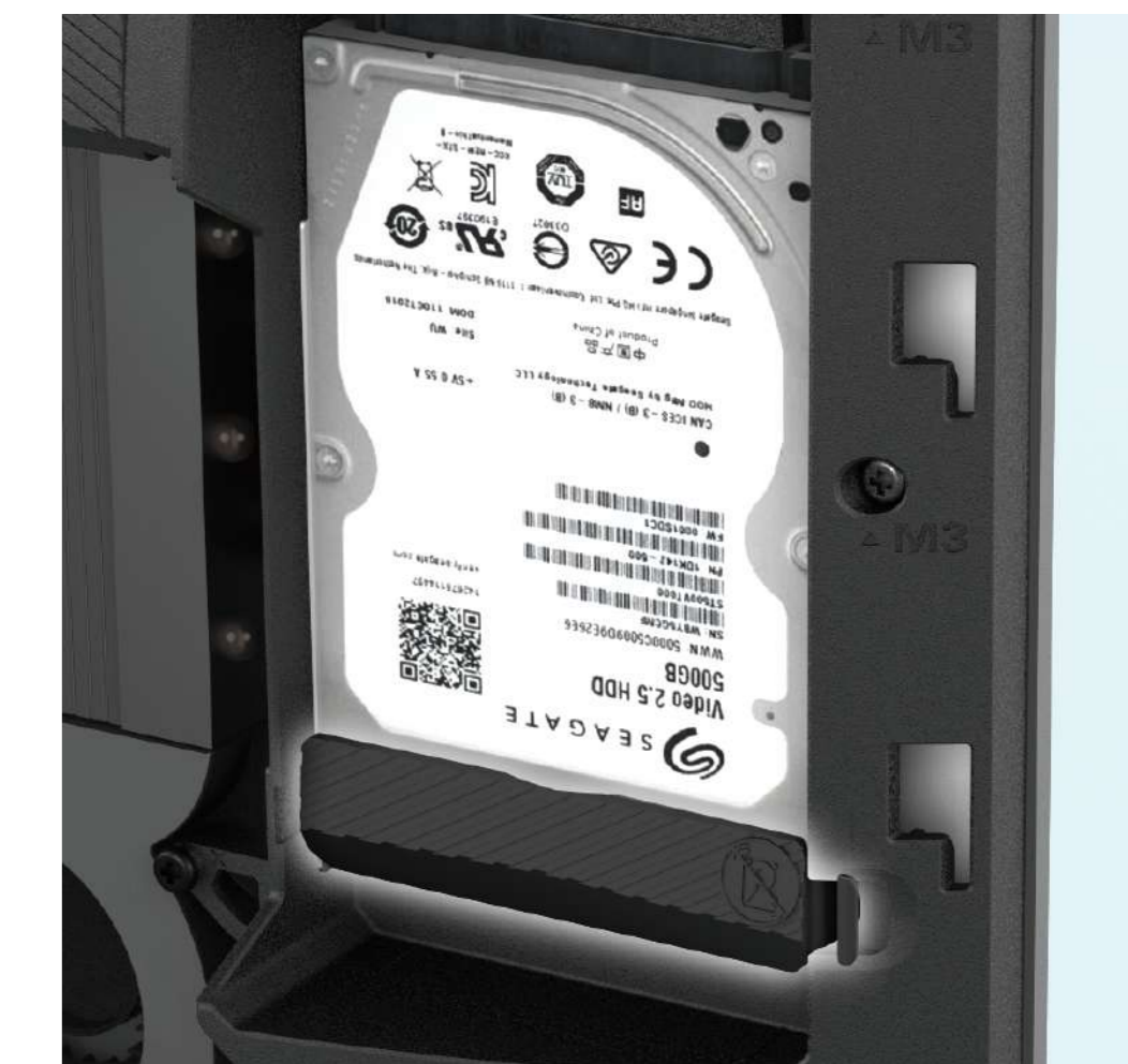
Exclusive shock proof clip, keep HDD from vibrating.
